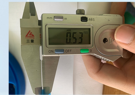
10. Measure the lower, middle and upper thickness without error Ultra and 0.03mm can be
